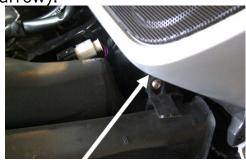
7) Press at arrow and slide duct forward.
